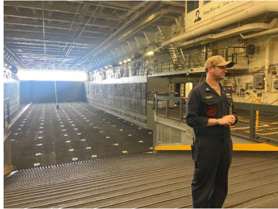
USS San Diego (LPD-22) briefer showing the stern opening area that literally allows the sea to enter the vessel and be used to ingress and egress amphibious platforms.
